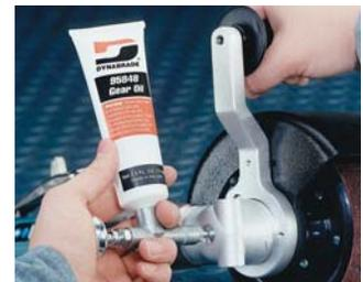
**NOTE:** For non wick-type lubrication systems, use 95542 Gear Grease.
