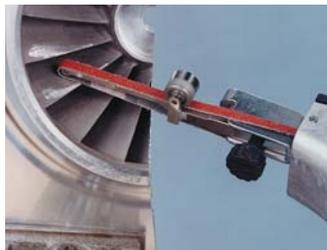
*Efficiently rework turbine blades with specialized contact arm.*
