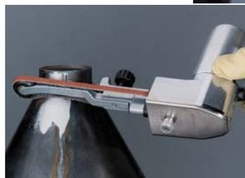
Slack of abrasive belt is used to efficiently polish radiused area.
