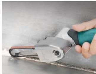
*Ideal for blending stainless steel and grinding right angle welds.*
