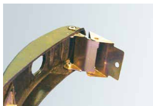
Composite material latch for wheel cover
