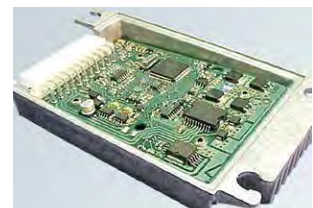
Automotive die-cast chassis with PCB
