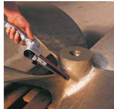
**Caution: comply with the speeds recommended by component and abrasive manufacturers.**
