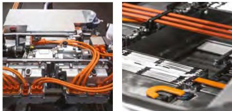
During the **assembly of components exposed to high voltage such as busbars and harnesses**, using insulated tools is one of the many important steps to protect from electrical shocks and damages:
