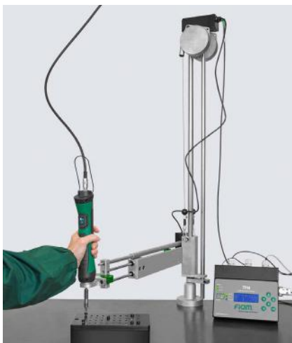
Cartesian arm with a position monitoring device.
