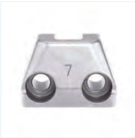
Die 7 For processing aluminium and stainless steel 600 N/mm 2 from 5 - 7 mm
