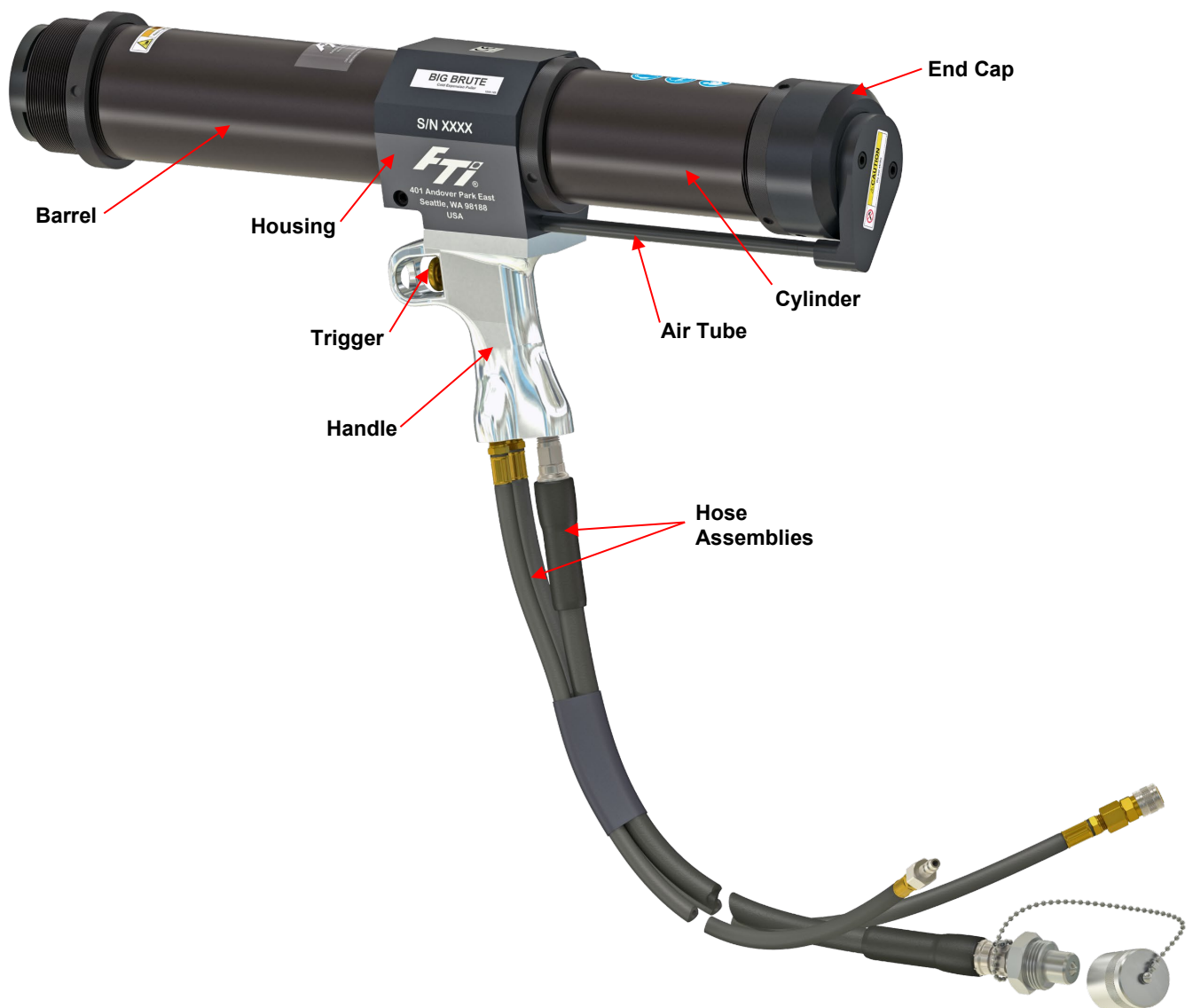
Figure 1.3-1 Big Brute Puller Unit Parts
